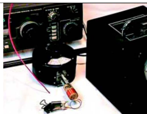
Use a calibrated receiver to monitor the dip meter's exact frequency while a crystal is "dipped"
